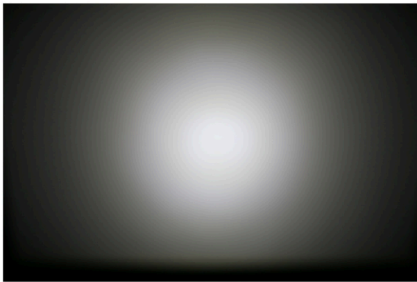
Spread Pattern - Medium Optic (32°)
