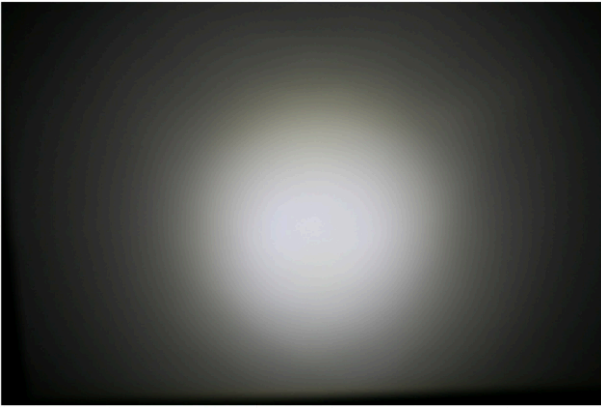
Spread Pattern - Spot Optic (24°)
